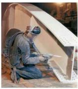
In the Arcspray process, two electrically charged wires are driven and guided so that they converge at a point and form an arc. An air nozzle atomises the molten metal produced and projects it towards
